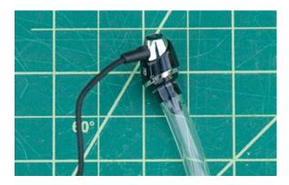
Make sure the tubing has cooled completely, and cut the tubing as straight as possible. Leave at least  $\frac{1}{4}$ " (6mm) past the end of the post.
