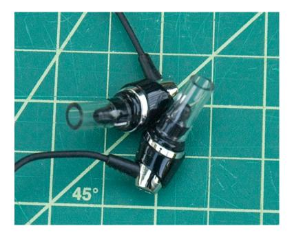
You don't have to take your processors off to put on the ear buds. With a little practice, you can hold your processor and T-mic in place on your ear, and gently push the tubing onto the T-mic. Don't force it on; it only needs to be on tight enough to hold the weight of the ear bud.
