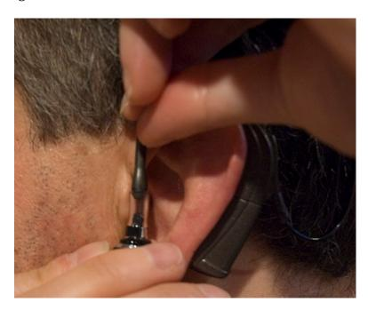
Put the ear bud on so the wire doesn't interfere with anything. I like to have the wire exit towards the front.
